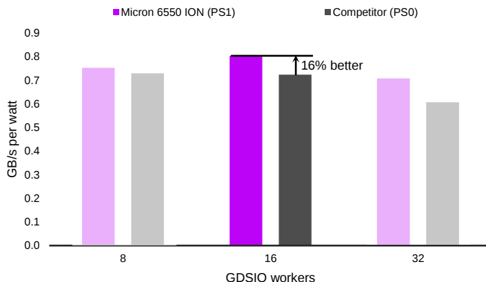
Figure 11: 1MB transfer power efficiency (GB/s per watt, higher is better)
