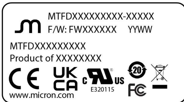
Figure 16: Embedded USB Label Structure
