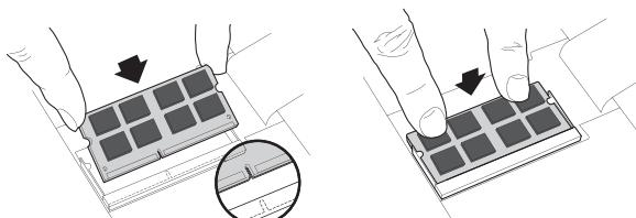
Firmly push the SODIMM/CSODIMM in at a 45-degree angle, and then push down until clips snap into place. When it is fully seated in the slot, one-sixteenth of an inch or less of the gold pins will be visible.
