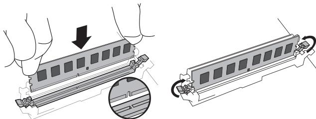
Using firm, even pressure, push UDIMM/CUDIMM into slot until clips snap into place. Do not assist clips.
